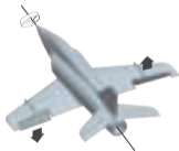
Aileron turn left during flight Aileron correction diagram
