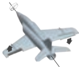
Aileron turn right during flight Aileron correction diagram
